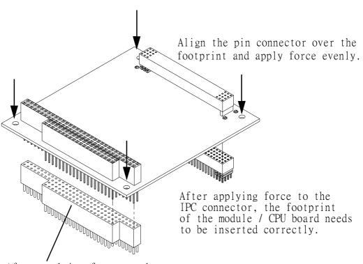
After applying force to the connector, the footprint of the module / CPU board needs to be inserted correctly.
