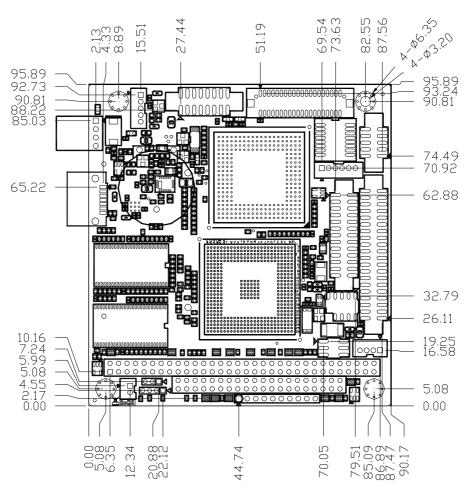
Figure 2.3 Board Dimensions Layout (Component Side)
