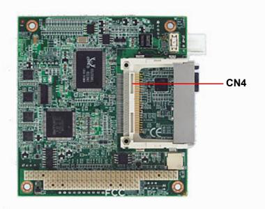
Figure 2.2 Jumper and Connector Layout (Solder Side)
