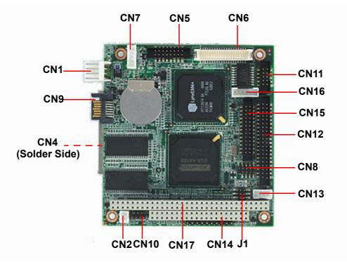
Figure 2.1 Jumper and Connector Layout (Component Side)
