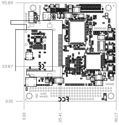
Figure 2.4 Board Dimensions Layout (Solder Side)
